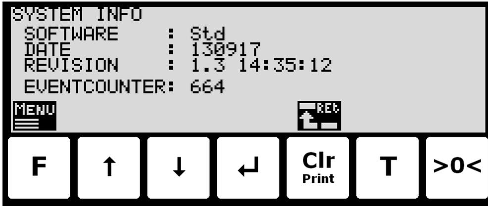
In this screen program identification (consisting of software name, date and revision) and the event counter is shown.
