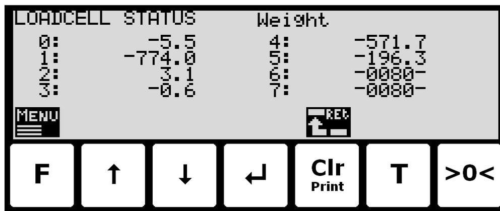
In this screen the actual reading from each loadcell is shown.
