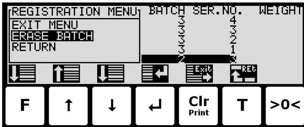
To erase the currently selected batch and all older batches select the “**ERASE BATCH**” menu item and press this will invoke the **DELETE BATCH** confirmation screen.
