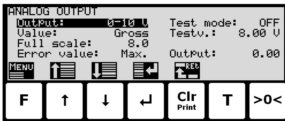
In this screen analog output parameters are shown and can be changed. A cursor (inverted text) indicates the currently selected parameter.
