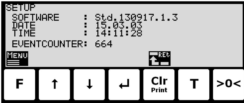
In this screen the software version, actual date, actual time and event counter is shown. The keys are used as follows:
