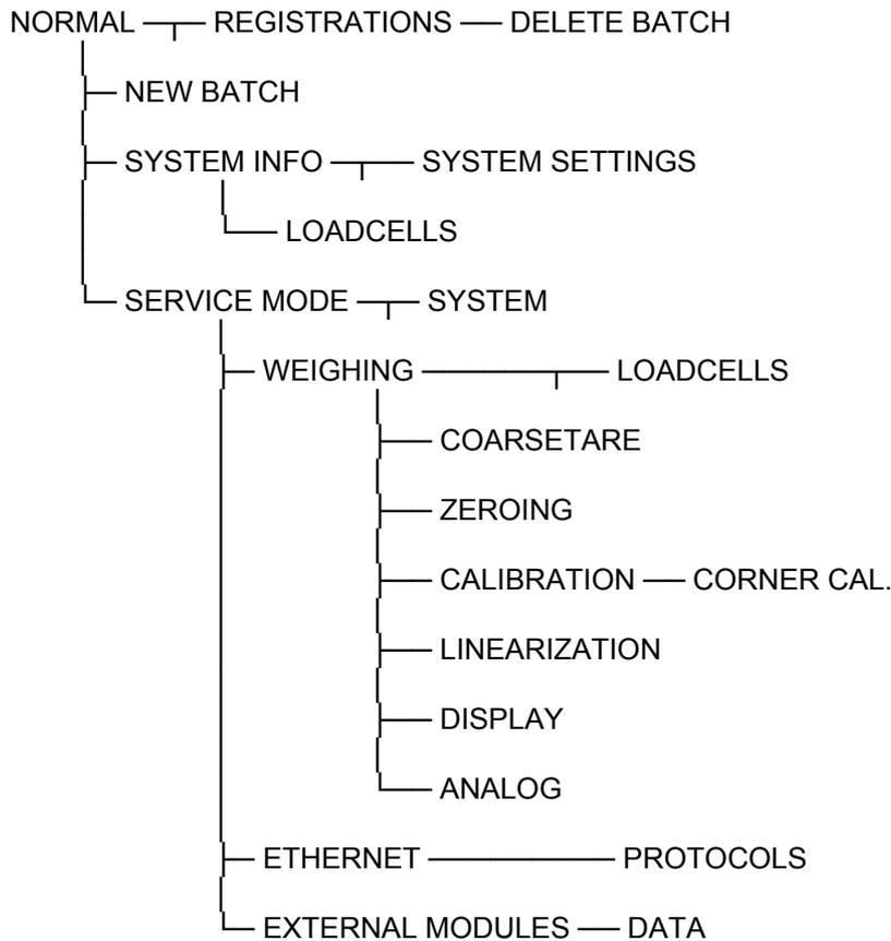
During normal use it is only necessary to use the **NORMAL** screen. The other screens are used during installation and calibration and registration check.
