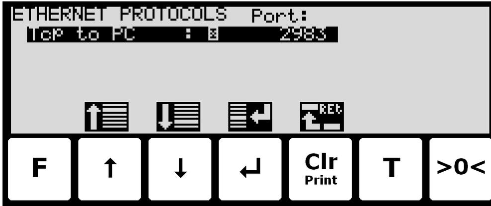
In this screen the different Ethernet protocols are shown and can be changed. A cursor (inverted text) indicates the currently selected protocol.
