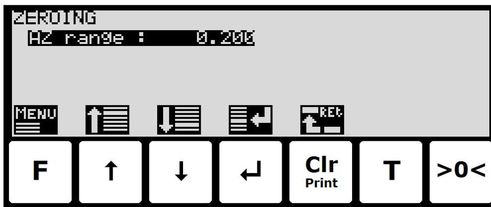
This screen is used to enter the zero tracking (autozero) range.
