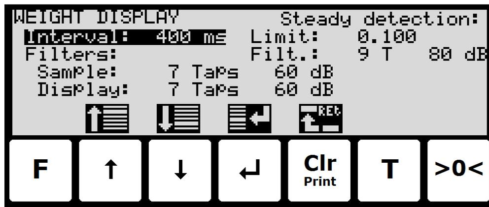
In this screen weight display parameters are shown and can be changed. A cursor (inverted text) indicates the currently selected parameter.
