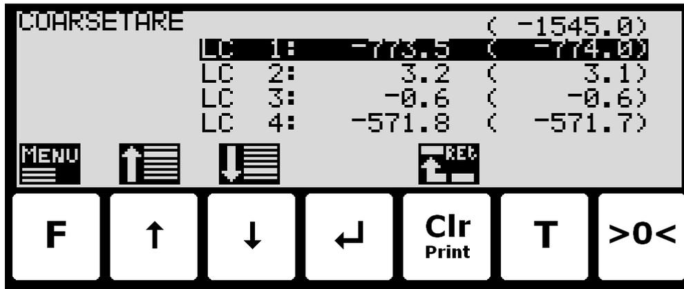
In this screen the coarsetare values and actual signals for each loadcell is shown.
