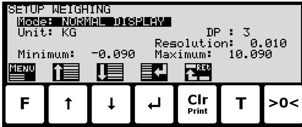
In this screen weighing parameters are shown and can be changed. A cursor (inverted text) indicates the currently selected parameter.
