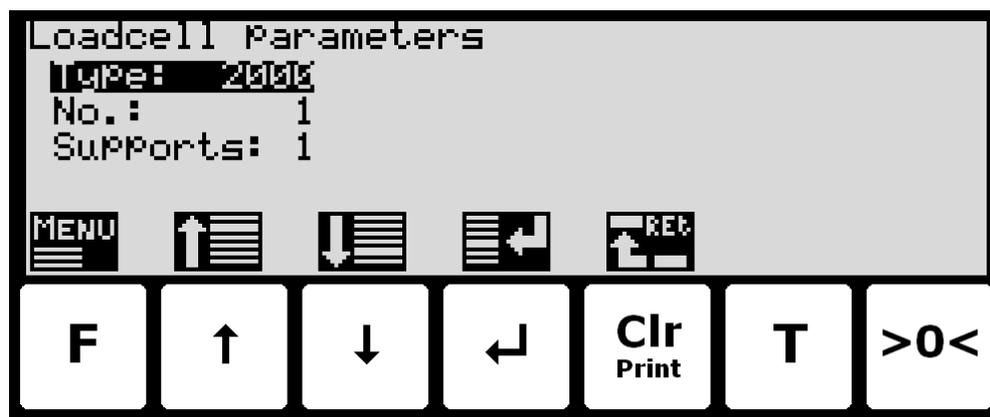
In this screen loadcell parameters are shown and can be changed. A cursor (inverted text) indicates the currently selected parameter.
