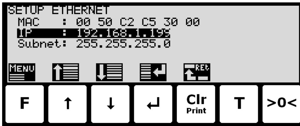
In this screen the different Ethernet parameters are shown and can be changed. A cursor (inverted text) indicates the currently selected parameter.
