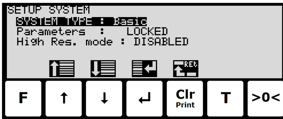
In this screen the system parameters are shown and can be changed. A cursor (inverted text) indicates the currently selected parameter.
