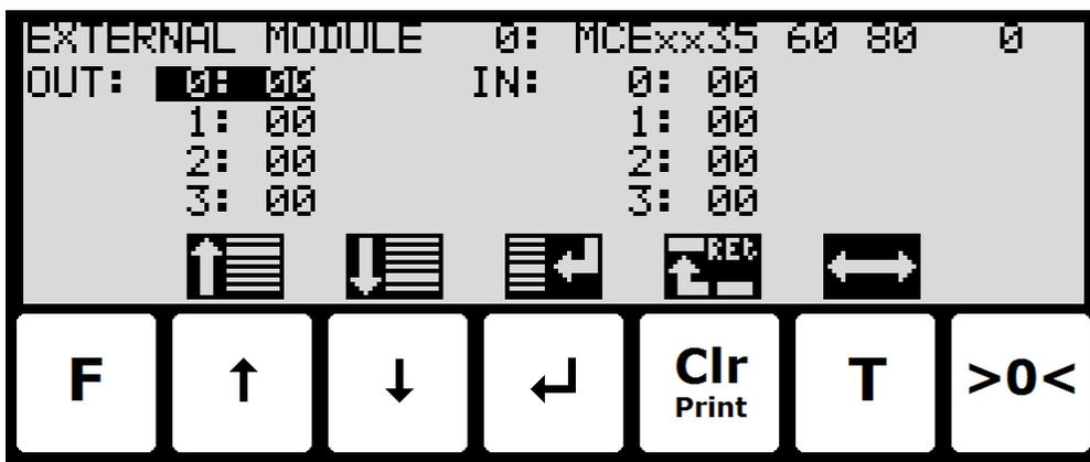
This screen will show the data sent to the external module (*OUT*) and the data received from the external module (*IN*).
