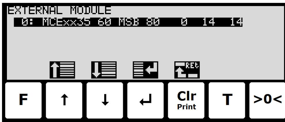
In this screen the external module is shown and can be changed. A cursor (inverted text) indicates the currently selected module. With this version of the software only one module can be installed.
