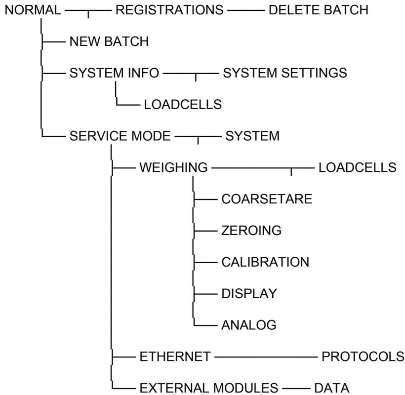
During normal use it is only necessary to use the **NORMAL** screen. The other screens are used during installation and calibration and registration check.
