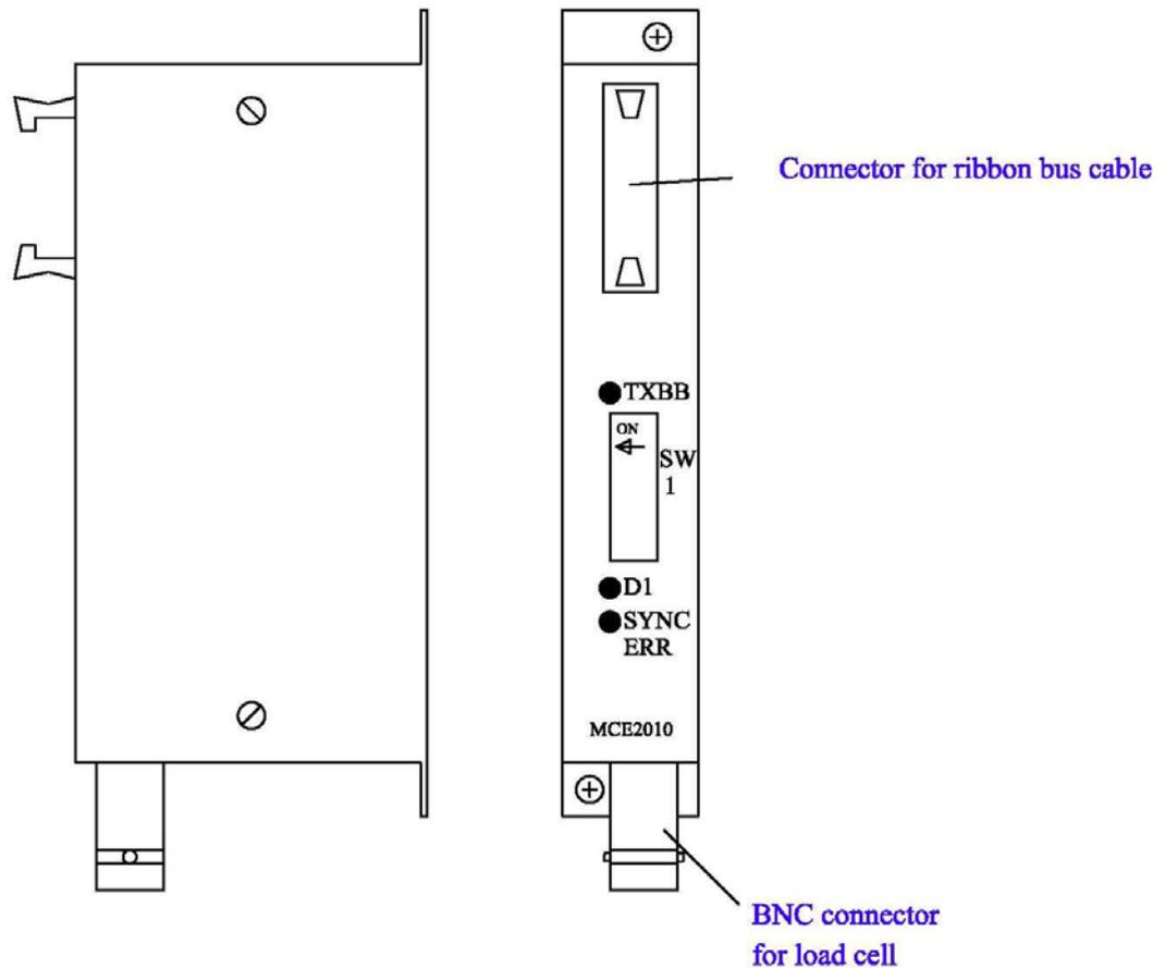
The load cell modules are connected to each other using the supplied cable (10 pole ribbon cable). The TE67X000002029 analog module is connected using the same cable.
