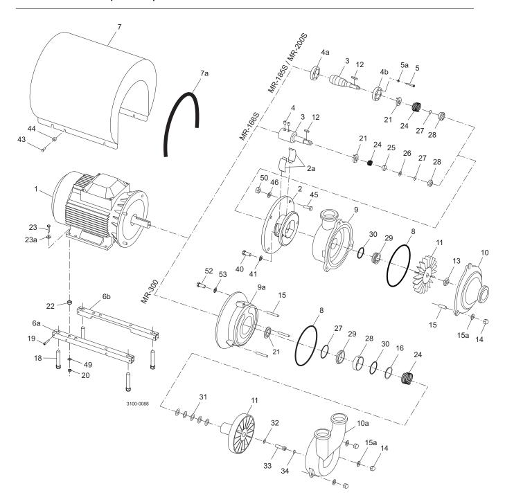
The drawing shows the MR-185S -200S, sanitary version. The items refer to the parts lists in the following sections
