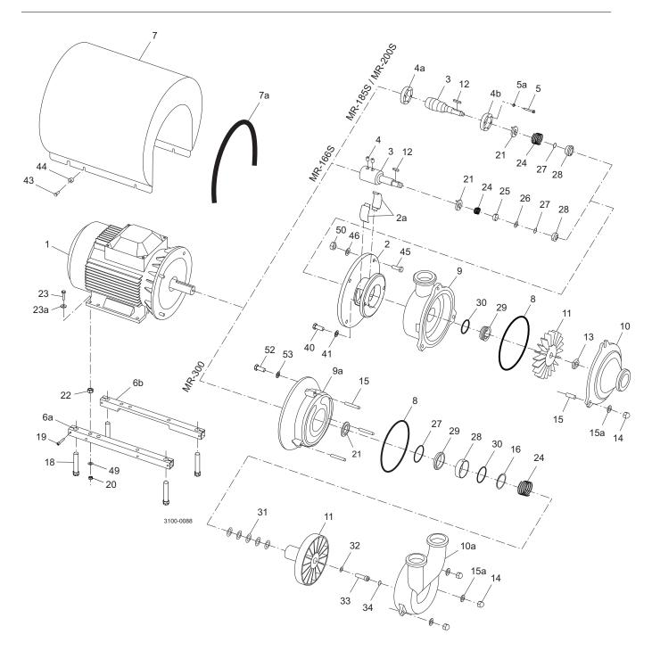
The drawing shows the MR-166S, sanitary version. The items refer to the parts lists in the following sections.
