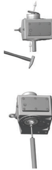
Figure 3-5: Removing the factory-fitted closing cap
