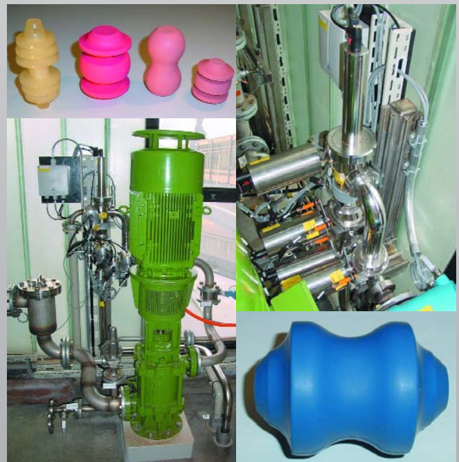
SMV pig launching station
